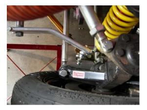
6. Install the 3/8" heims into the hexagonal turnbuckles and then install them between the ends of the swaybar arms and the lower control arms using the included short bolts and nuts. Each bar stock will use one right hand thread heim and one left hand thread heim. The left hand thread heim goes into the end with the score mark on the outside. The hexagonal turnbuckles should be left "loose" so they can be adjusted.
