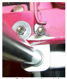
You may find you need to grind or cut some oil cooler bracket mounting out of the way on the inner side of the frame as shown above.
