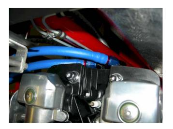
3. Install the water pump on the flat plate of the water pump bracket, and then bolt the bracket into the top two holes of the driver side upper control arm mount. Be sure the water pump outlets are all pointed toward the passenger side of the car. If not, the bottom of the pump can be removed and the outlets rotated correctly.
