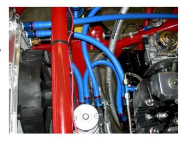
6. Install the adapter and temperature gauge probe in the radiator. Run the lines back to the interior of the car and install the water temperature gauge. One good location is where the tach recall used to go, as shown to the right. The tach recall can be placed on the side panel below the fan switches.
